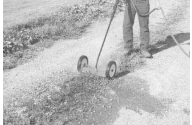
Weeds need to be within 6 in. of nozzle in order to be killed, since heat dissipates quickly into the air.
