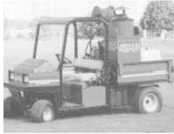
System heats water to 280 degrees F and then sprays it out through a nozzle.
