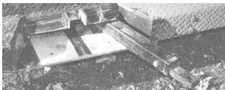
Hitch slides back and forth for easy hookups. Locks in place at center for towing.
