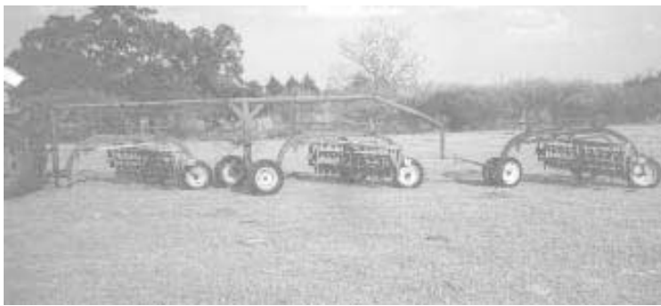
Home-built triple rake hitch lets Chudej hook three 9-ft. side-delivery rakes together to cover 27 ft. at a time. Hitch is made from heavy-wall oil field drill stem pipe.
