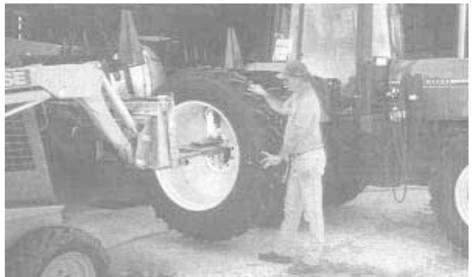
"Dual Doohickey" is designed to mount on the forks of any skid steer loader.
