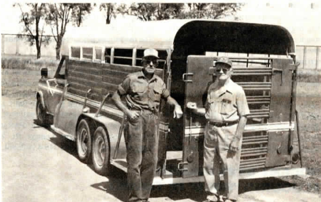
Scott cut off the rear end of a 4-WD IH Scout pickup leaving the front drive axle to power the horse trailer.
