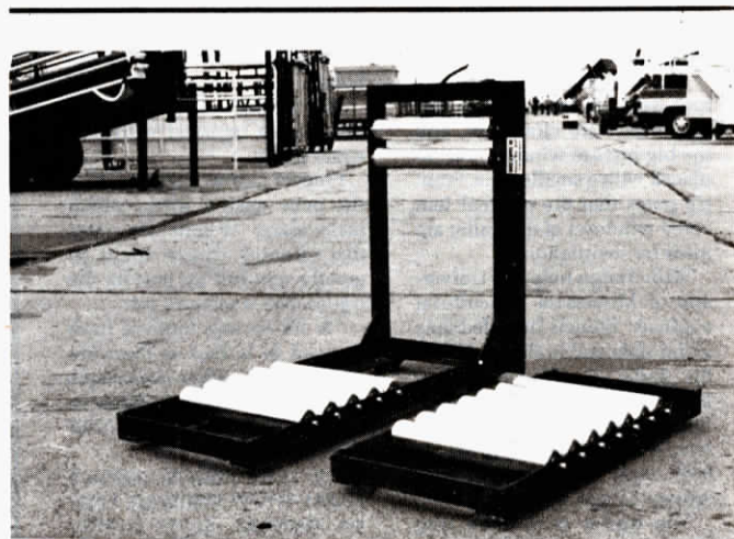
As tower wheels move onto rollers, they spin and thus prevent tower from moving forward. This causes misalignment and automatic shutoff.
