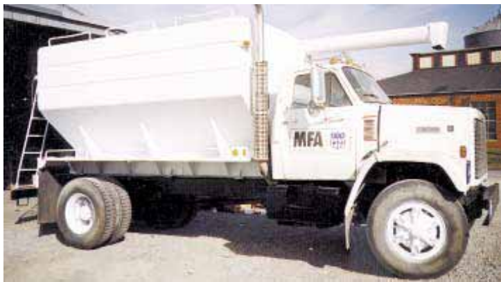
Only a complete sandblasting and thorough cleaning of the bare metal to eliminate soluble salts and other contaminants can ensure a long-lasting paint job like this truck received, says Deardorff.
