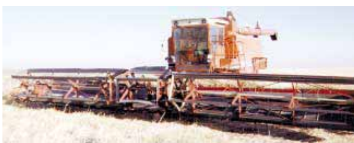
Richard and David Pope used three Versatile pull-type swathers to make a 40-ft. header, which they mounted on their IH 1480 self-propelled combine.
