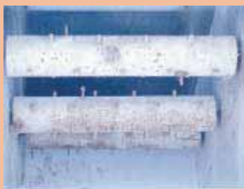
After forage is dried a little, finger rollers at the bottom of the compartment move the material to the next lower compartment.
