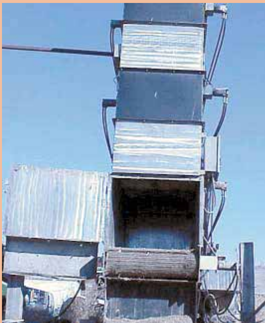
Forage is put into top compartment and then works its way gradually down through lower compartments until it reaches the bottom, dry and ready for storage.
