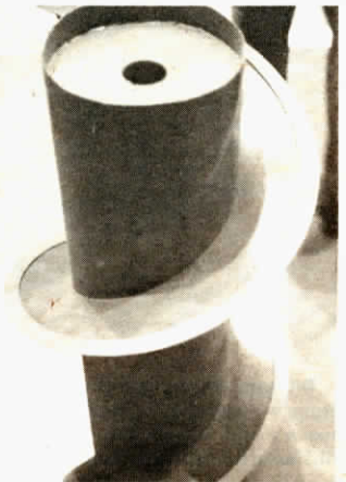
Metal strips weld to outer edge of auger fighting.
