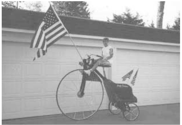
The driver never has to pedal this high-wheeled tricycle. All the work is done by an 8 hp gas engine which belt-drives a 3-speed transmission off a riding mower.
