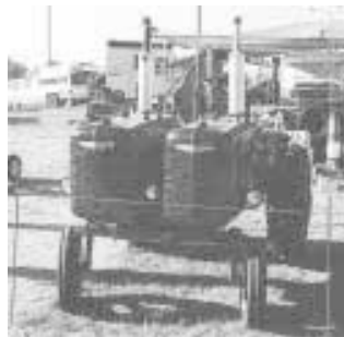
Either tractor's motor and transmission will work separate or both will work together at the same time.
