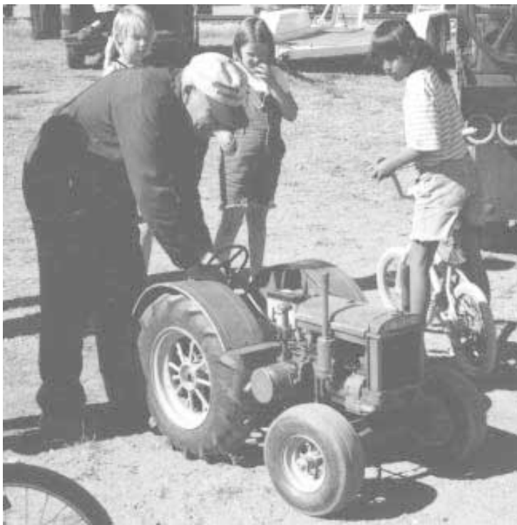
Retired machinist William Ives built this mini 1936 Deere "D", scaling it down to one-third size by taking measurements from the real thing.
