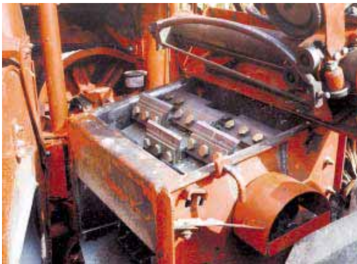
After conversion, cutterhead is fitted with 27 knives and a "kernel cracker" that requires virtually no horsepower to operate, according to Eder.
