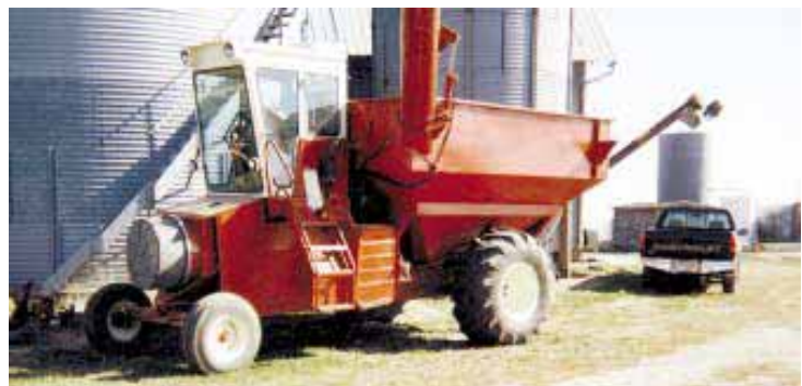
Vaessen patterned his home-built 400-bu. grain cart after a commercial rig. His biggest cash outlay was for the 14-in. dia. unloading auger.
