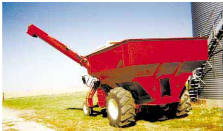
Vaessen patterned his home-built 400-bu. grain cart after a commercial rig. His biggest cash outlay was for the 14-in. dia. unloading auger.
