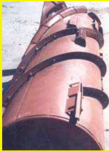
Makeeff adds flighting to back half of rotor to keep crop material flowing through combine.
