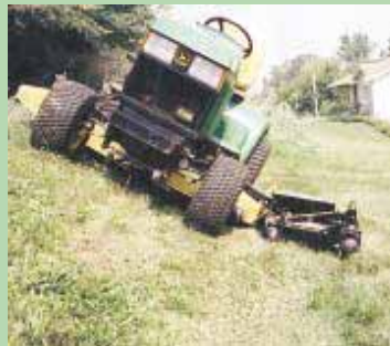
Add-on Flex-Deck flexes up 45 degrees and down 8 degrees.
