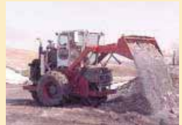
Tractor can be fitted with dozer, front-end loader, or any other attachment.
