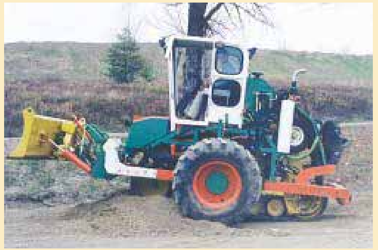
New tractor is powered by single rubber track at center. Wheels on either side are primarily for steering and stability.
