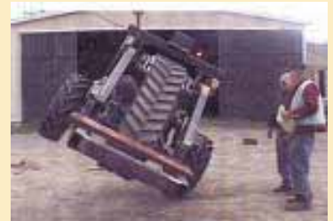
During testing, machine was tilted 45 degrees without tipping.
