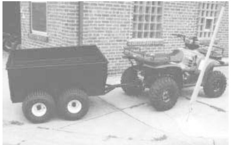
Tandem axle suspension gives ATV trailer plenty of carrying capacity for farm chores.
