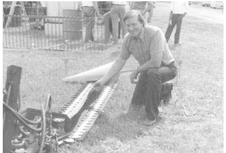
Willard Pearson installed this prototype "Chain Sickle" on a 7-ft. hay mower. It used conventional sickle sections on a specially-designed linkage system.
