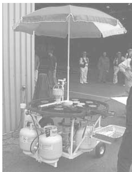
Batter is measured and dropped automatically onto a large round griddle which is rotated slowly by a 120-volt AC motor. An umbrella provides shade for the operator.
