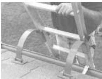
Brackets slide onto the ladder side rails and arch over edge of roof to put weight of ladder directly on top of roof.
