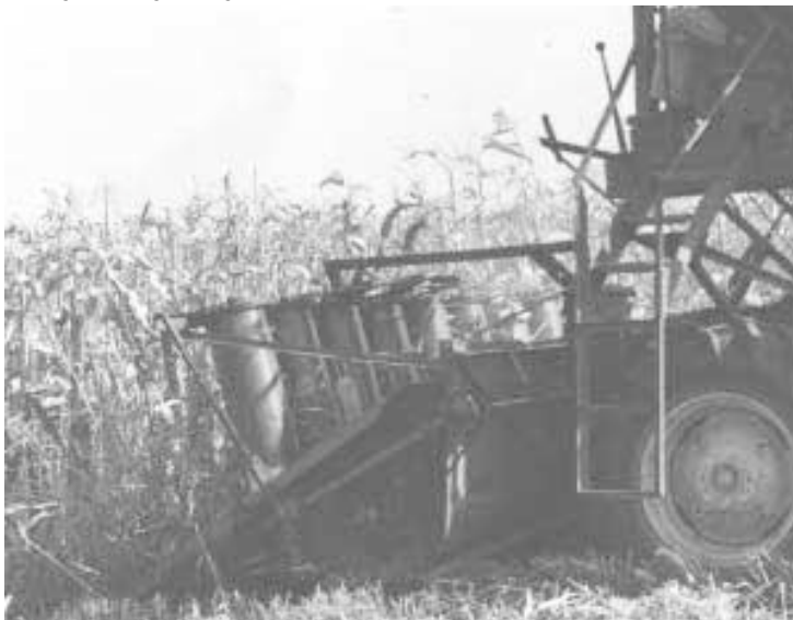
Fingers came out to grab stalks and pull them into the combine, then retracted to release them into the machine.
