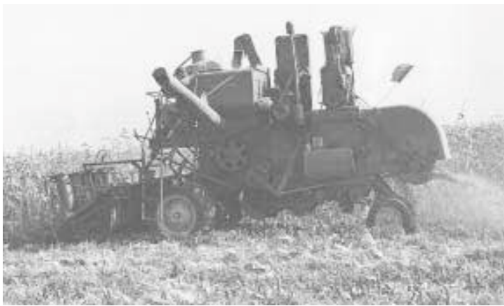
Back in the 1950's a pair of Illinois farmers fitted a conventional grain header with rotating vertical gathering drums equipped with retractable fingers.
