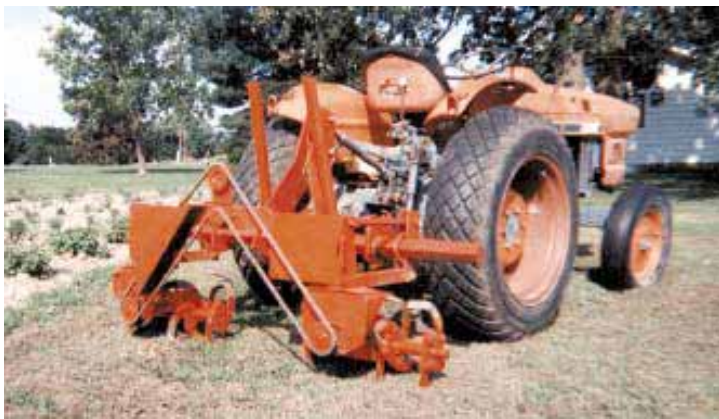
Kinney used two walk-behind tillers to build his tractor-mounted rotor tiller. He uses the 2-row tiller behind a Kubota 31 hp tractor with its wheels set in for 40-in. spacing.
