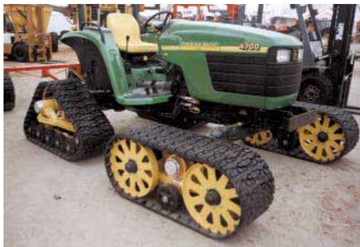
New Mattracks track conversion system is available for smaller 4-WD tractors. It consists of four separate sets of 16-in. wide tracks.
