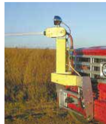
Fire-fighting nozzle mounts on front of pickup bumper and is controlled by a joy stick inside cab. Note spotlight on top of nozzle.
