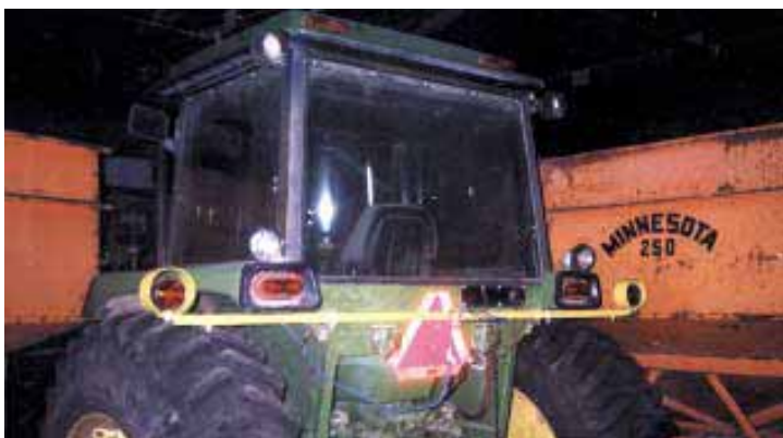
Telescoping light bar mounts on back of tractor or on the back of wagons or other equipment.
