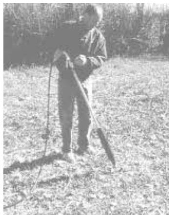
To use new post hole digger you first hook it up to a garden hose. It takes less than a minute to "dig" a 4-ft. post hole that's 4 in. in diameter.
