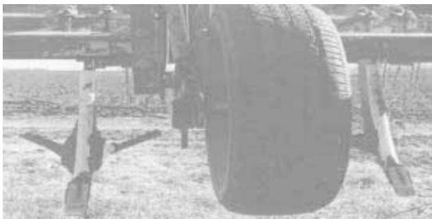
Made from anti-stick poly, "Superslide" protectors prevent dirt and trash from sticking to subsoiler shanks. They also prevent shank wear.
