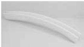
Shank protectors are about 2 ft. long and 2 in. wide and have a 1 1/2-in. deep hollow channel that allows them to simply slip tight over the shank.
