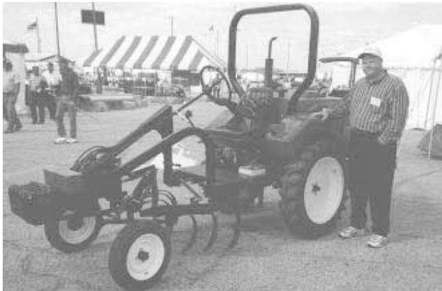
MHP (Mobile Hydraulic Platform) has modern features such as a diesel engine, hydrostatic transmission, independent hydraulics and a rear pto.
