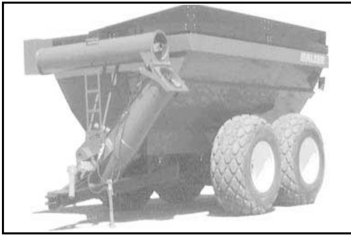
Balzer's new "Field Floater" grain cart can be equipped with either walking tandem axles or independent triple axles. Hydraulic cylinders keep the steerable axles parallel to each other and allow them to follow the tractor's direction.
