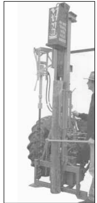
Post pounder is equipped with a small auger. Controls are on back for easy access from the ground.
