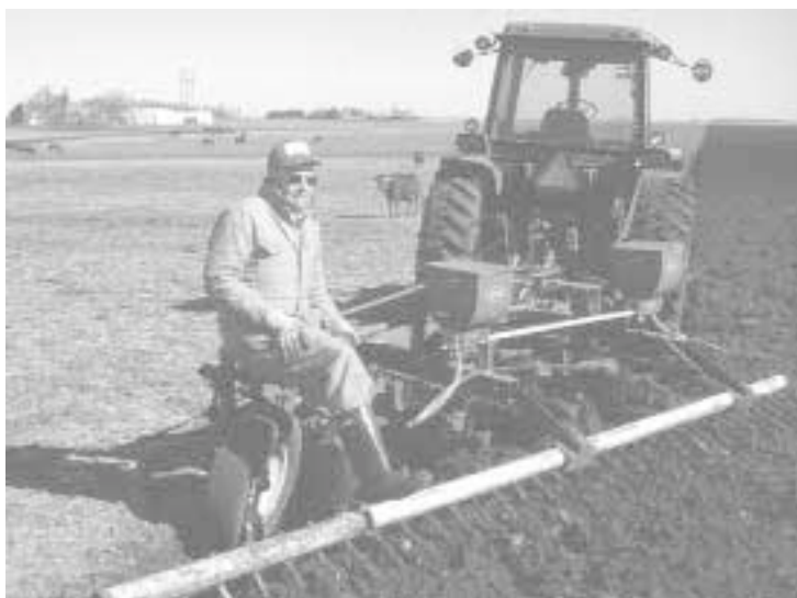
By mounting Gandy seed boxes on his moldboard plow frame, Dick Thompson of Boone, Iowa, can broadcast winter rye onto fall-plowed ground.
