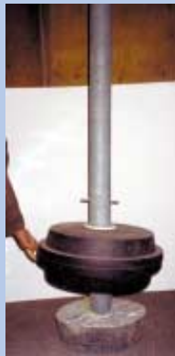
A 65-lb. concrete weight is fixed to bottom of post, with a float mounted above it.
