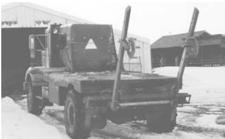
Back end of truck is equipped with bale-handling arms that unroll bale on ground. Behind the cab is a homemade 40-bu. hopper that can be removed with the arms.
