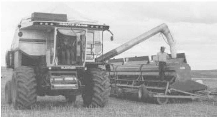
A Gleaner combine is used as a drill fill. It has a flexible plastic down spout at the end of the unloading auger and also a specially-designed tarp over the tank.
