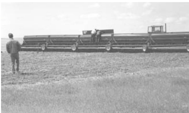
Arnal's 87-ft., hoe drill is made up of 6 Case-IH 7200 14-ft. drills hooked together with a custom-built transport hitch. He can plant over 160 acres without having to refill.
