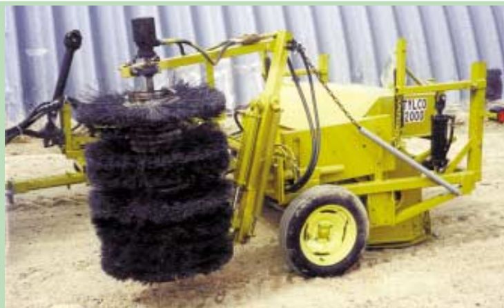
Fence sweeper is equipped with rotating brush and chopper-mower to sweep off weeds that collect on fences.
