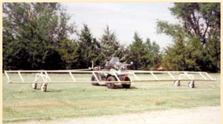
Wick wiper is built in two 20-ft. sections that each ride on a pair of in-line castor wheels. Wiper can be hydraulically lowered to within 3 in. of ground or raised as high as 6 ft.
