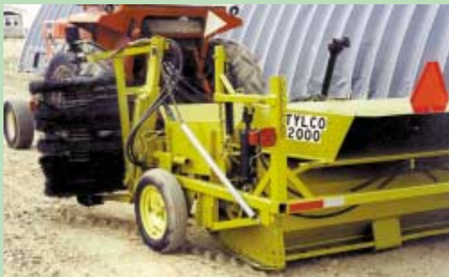
As driver moves forward, brush sweeps weeds into chopper which then blows them out the back.
