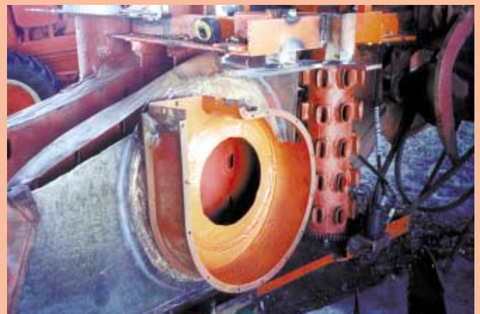
The only moving parts in the header are a centrifugal fan and a rotating drum that extracts cotton from the boll.
