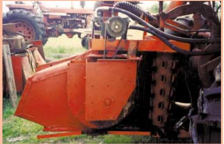
Randy Thompson of Sycamore, Ga., designed and built this picker that pulls cotton bolls off plants without pulling plant parts through the machine.
