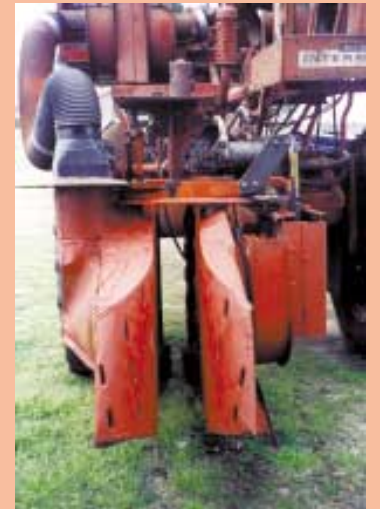
Compared to conventional pickers, the new header weighs less per row, requires less power, and results in cleaner, better quality lint, says Thompson.
