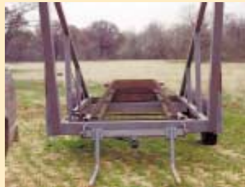
Rig is equipped with a pair of hydraulic-operated forks on front and a conveyor chain floor. Trailer swings out to side of pickup to load bales.
