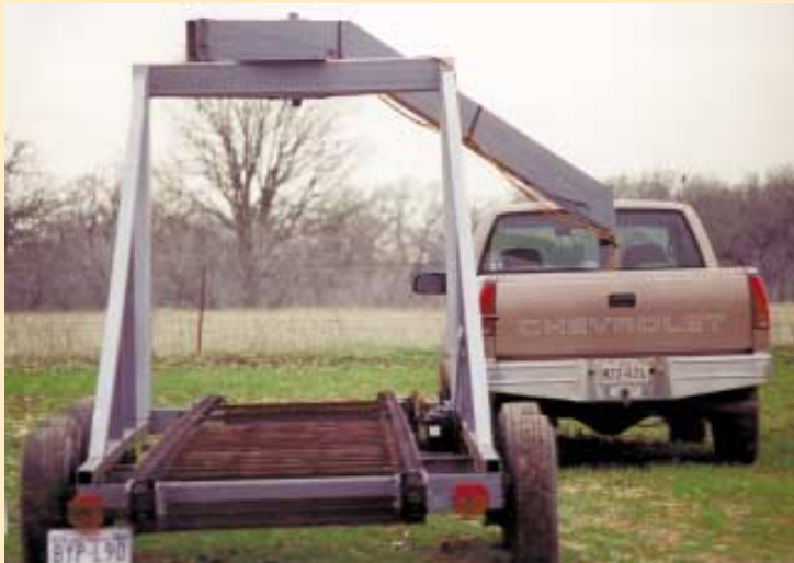
Bales can be unloaded off back or front using conveyor chain.
