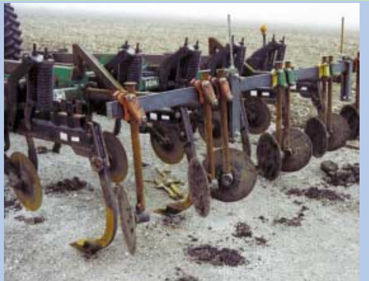
To level the ground behind his chisel plow, Robert Dunton mounted a disc behind each shank. The discs break up dirt chunks and spread out dirt behind shanks.
