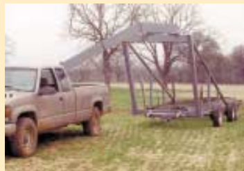
Bales are placed onto front part of trailer and then moved back just far enough to make room for next bale.
