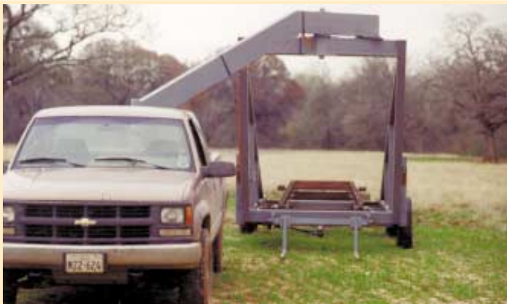
Eiland uses his 3/4-ton 4-WD pickup to pull his self-loading, fifth wheel bale hauler.
