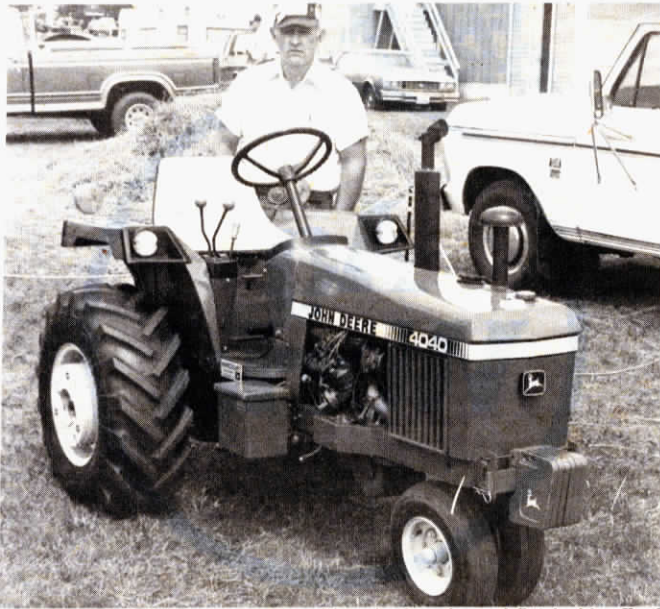
Paulsen's "mini" 4040 is powered by a Pinto 4-cyl. engine and fitted with a Ford Fairlane transmission.
