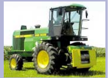
To get more capacity from his Deere 5400 SP forage harvester, Klassen replaced the J-knife cutterhead with a 64-knife drum.
