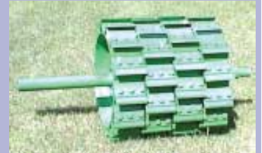
Klassen now manufactures drums with 40, 56, and 64 knives for the older 5000 series Deere harvesters.
