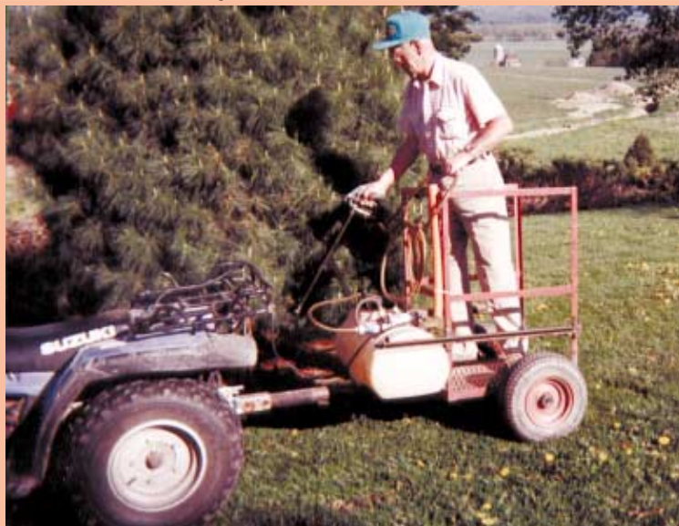
Don and Craig Winship made a spray "chariot" to pull behind their ATV. "It cut our spraying time by two thirds," says Craig.
