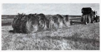
Photo shows five bales just loaded off tag-along buggy and first bale of next load being kicked out of baler and onto empty platform.
