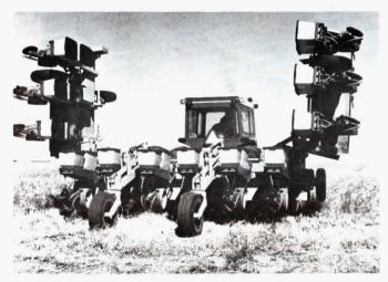
Center section is 180 in. wide, and each wing is 90 in. wide, for total width of 360 in. to accommodate 12 30-in. rows, or 10 36-in. rows.
