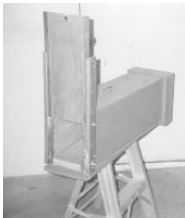
Sliding door on end of trap (right) is held up by the tip of a 1/8-in. dia. steel rod that runs back to ramp.
