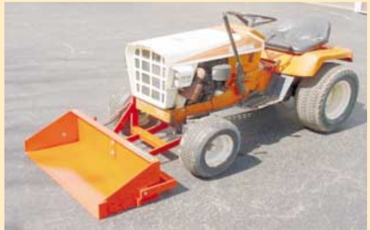
Johnny Bucket Jr. is designed for Simplicity and Bolens garden tractors with 8 to 20 hp. It's operated by pulling a dump trip cord.
