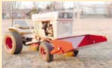
Bucket pins onto tractor frame using existing attachment mounts.
