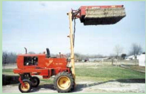
Two-stage mast can be used to stack square bales up to 14 ft. high.
