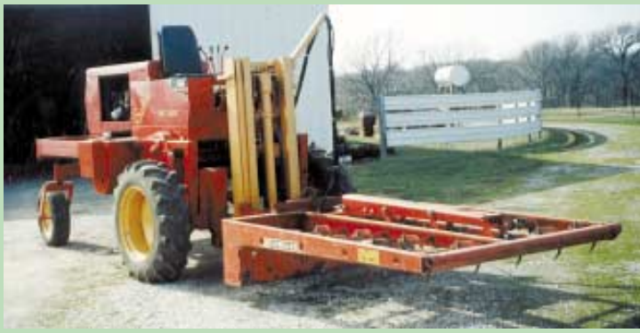
Sallee mounted a forklift mast on swather. He can fit it with a 10-bale Farmhand bale grabber, a 48-in. long bale spear, or simply use it as a conventional forklift.
