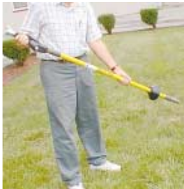
Unit requires an air compressor that can supply 175 to 185 cfm of air at 100 psi.
