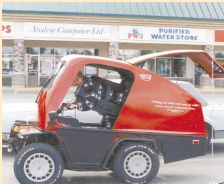
Cage can be covered by a fiberglass body with an electrically-operated rear entry door. Fitting the ATV with 14-in. car wheels allows it to run at highway speeds.
