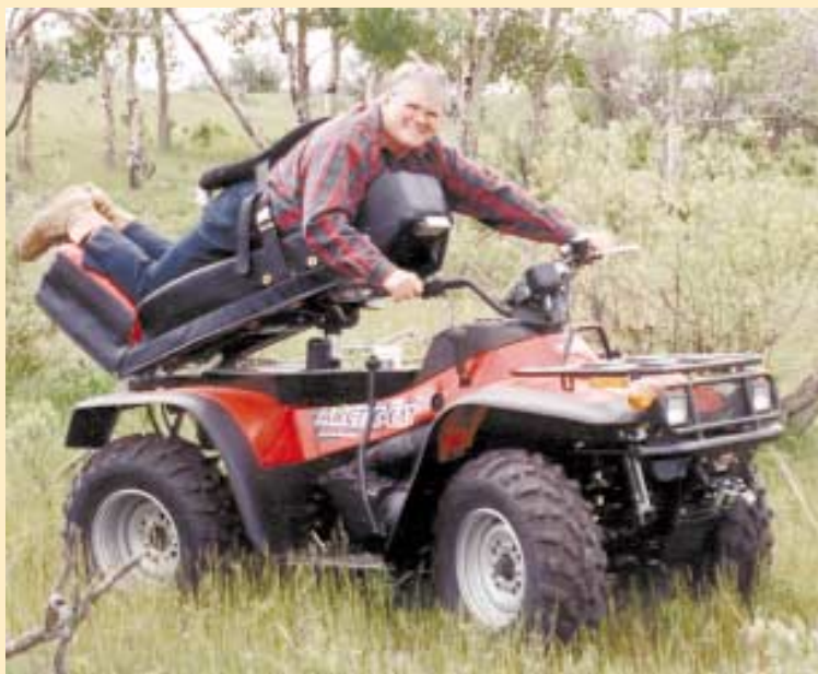
You'll save your back and also have a better view with this new full-length "seat" that's designed to lift a person up into operating position.
