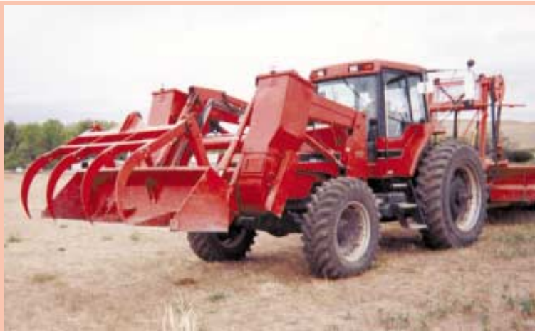
A feeder hopper mounts on each loader arm on Case-IH 7110 Magnum tractor. Each hopper holds about 400 lbs. of pellets.
