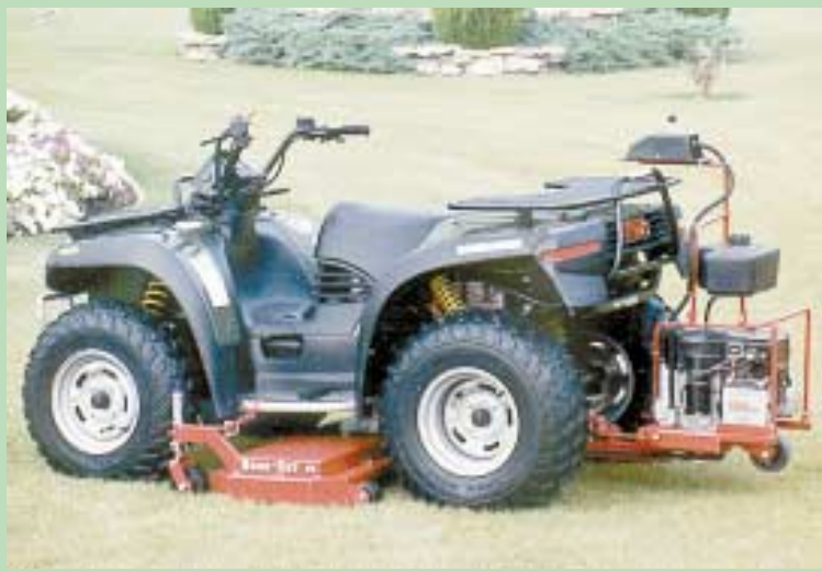
Kit comes with a 58-in. "mid-mount" deck powered by a 16 hp gas engine on back.
