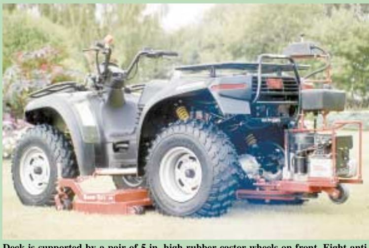
Deck is supported by a pair of 5-in. high rubber castor wheels on front. Eight anti-scalping wheels on back of deck prevent scalping on uneven terrain.
