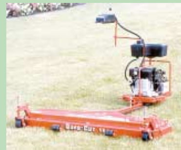
Engine platform connects to deck by bar that fastens to ATV.
