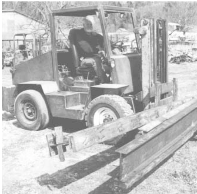
Clair Wilson used a 1974 Chevrolet 3/4-ton pickup frame to build this forklift.
