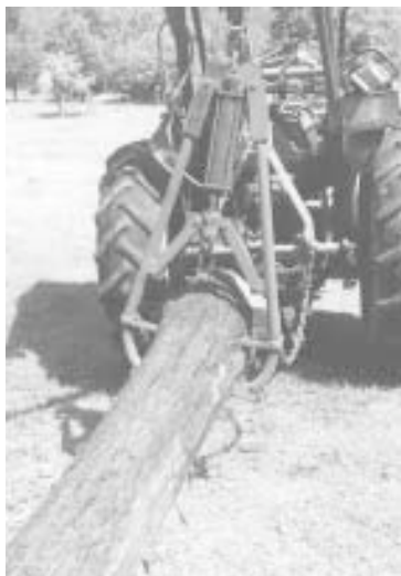
Log puller attaches to 3-pt. mounted boom. It consists of a pair of big steel “scissor action” tongs that are opened or closed by a 10-in. cylinder.
