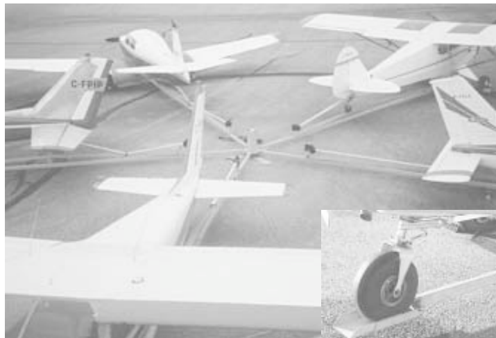
Rotating aircraft carousel holds five planes. It’ll fit only buildings with at least 70 ft. of open space. Inset photo at lower right shows how wheel fits onto ramp.
