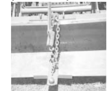
Temporary ball hitch attachment fits over lower lip of loader and is held in place by a chain that fits over a loader grab hook.
