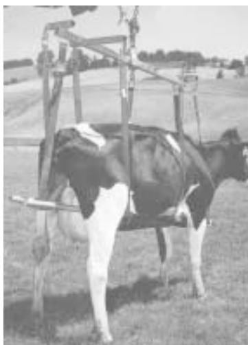
Lift is designed to hang by chain from a front-end loader.
