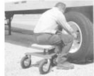
Triangular-shaped stool rides on three 8-in. pneumatic tires.
