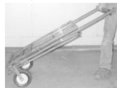
A pair of wheels lets you roll bench around like a 2-wheeled handcart.
