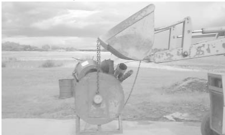
Scrap iron bin sits outside the Allard's shop until it's full. Chains hooked to front and back of bucket dump bin when bucket is dumped.
