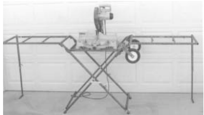
Bench consists of a drop center table with two heavy duty wings supported by adjustable folding legs. “You can use it in a lot of different ways,” says inventor Clint Birkeland.
