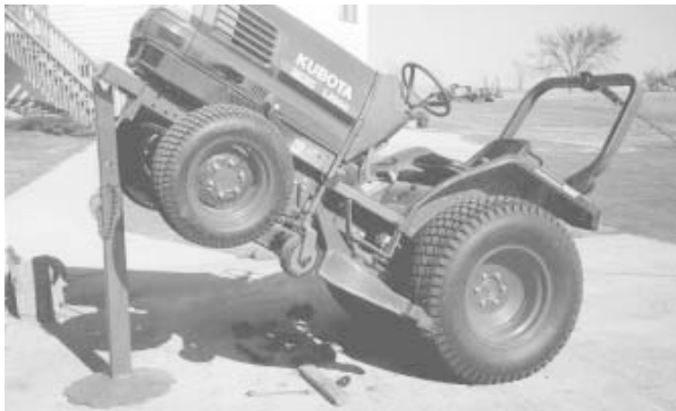
Tractor is anchored by a chain hooked to rollbar. Safety stand secures front end of tractor while it's up in the air.
