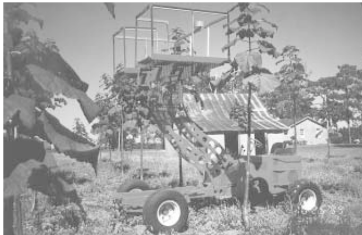
Thompson figured there probably wasn't a more stable machine than an Air Force bomb loader so he bought one and converted it into a pruning platform.
