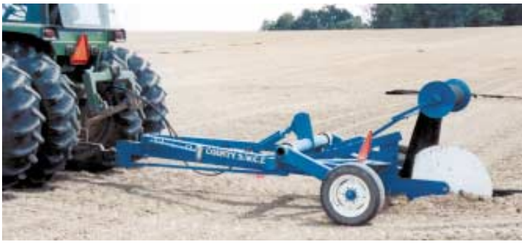
“Fabric plow” is equipped with a single large shank that digs a slot about 16 in. deep.
