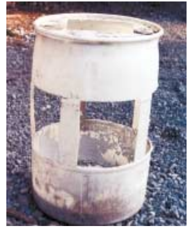
Five big holes are cut around the outside of a 55-gal. plastic drum, leaving strips between the holes.
