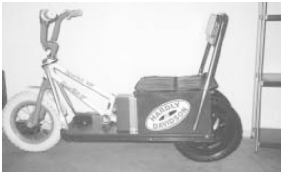
“Scooter is powered by a 12-volt battery and has two wheels on back.
