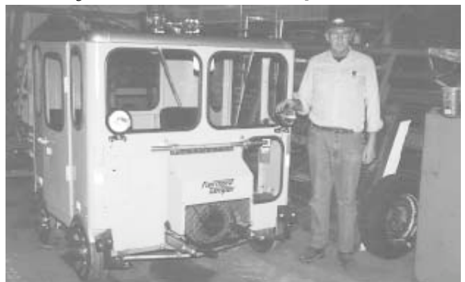
Hinds’s 6 by 8-ft. car is powered by an Onan 2-cylinder gas engine.
