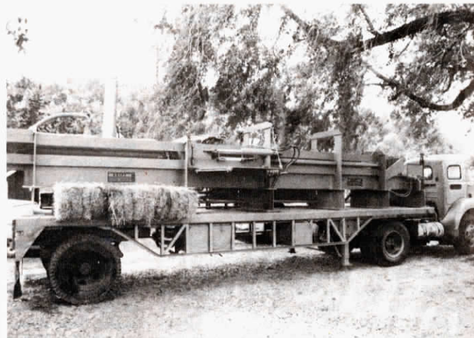
Containerbaler compresses up to 5 bales per min. "It could be designed to compress big round bales if anyone was interested," says Kraft.
