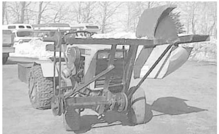
Stationary buzz saw was converted to a portable one that fits on front end of Hermanson's 10 hp Case garden tractor. He uses it to cut up three to four cords of wood each winter.
