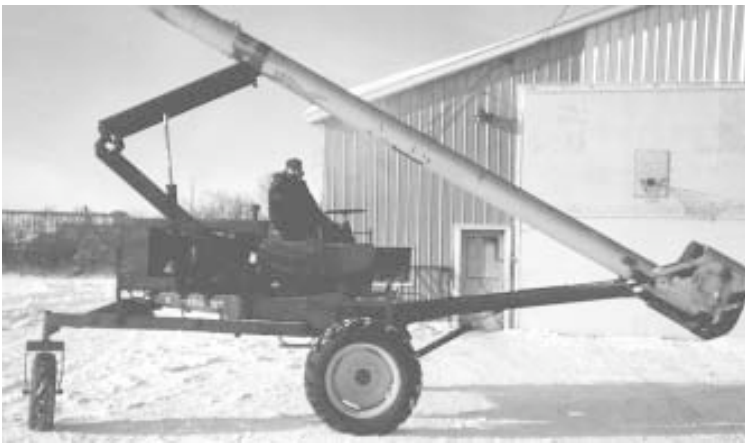
Toews combined a 50-ft. long, 10 3/4-in. dia. auger with an old Versatile 400 swather to make his self-propelled auger. "We can load 75 to 100 bu. a minute with it," he says.
