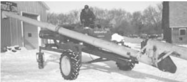
Self-propelled auger is highly maneuverable and moves grain quickly, says Toews.
