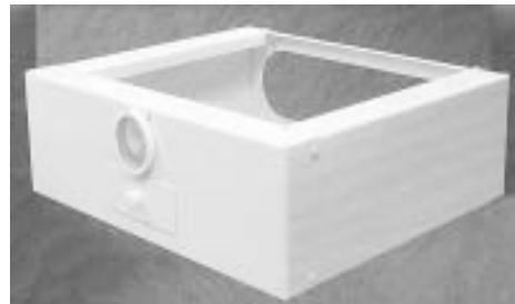
Air from dryer vents into unit through a heat-exchanging filter, and then outside the house. In cold weather, you open a slide gate to let clean, warm air into the house.
