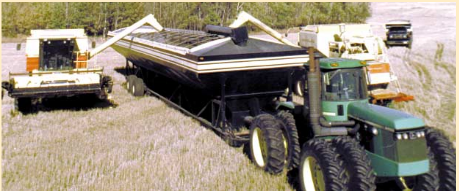
Measuring 65 ft. long, 12 ft. high, and 14 ft. wide, this giant grain cart holds a whopping 5,000 bu., or about 25 dumps from the Johnson's combines.
