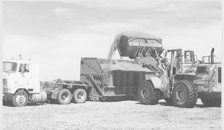
Another worker uses a loader tractor to load the piled silage into a side-dump semi-trailer.
