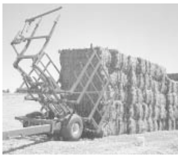
At the unloading site, a pair of cylinders are used to tip the trailer so the entire load stands on end.
