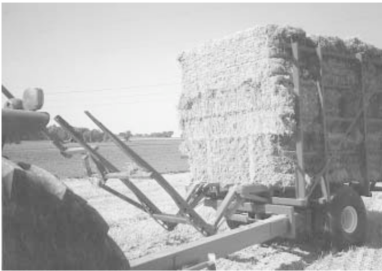
Pull-type unit is equipped with an offset hitch and has a hydraulic-operated loading arm on front that's attached to a pair of lift forks.
