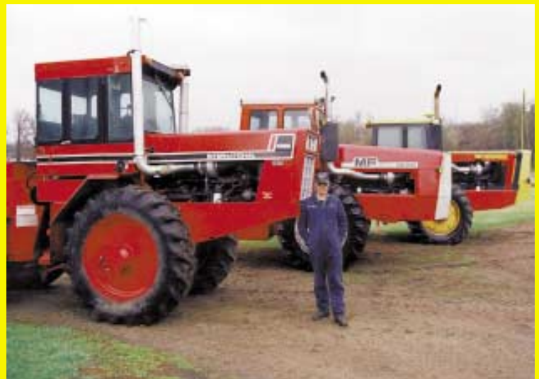
Keith Kjenner and four mechanics repower 4-WD tractors with Cummins 6-cyl. diesel engines. Photo shows just a few of the brands they work on.
