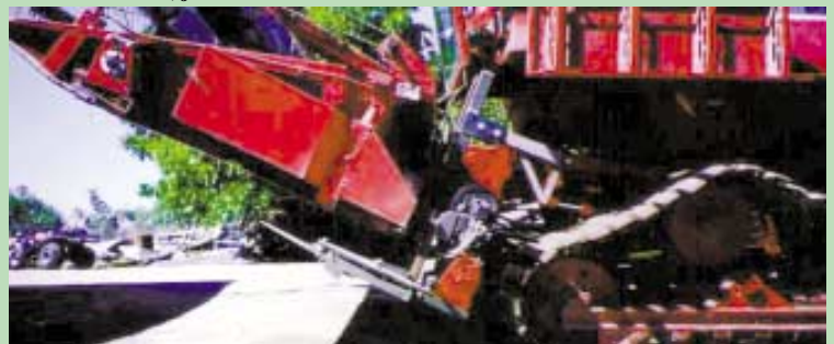
Hydraulic cylinders allow the cutting height of cutterbar to be easily adjusted so it doesn't run in the dirt.
