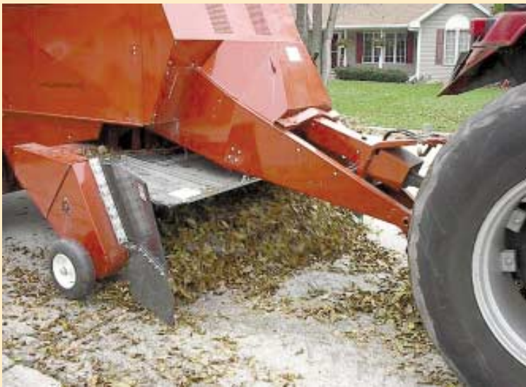
Leaves are funneled into bale chamber with the help of two side panels and a poly cover that mounts over baler pickup.
