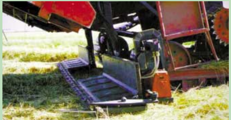
“Under head” stubble cutter provides a way to cut the straw stubble and clear it from path of combine. It consists of a sicklebar cutter with a draper windrower and fits under the header, just in front of the combine tracks.
