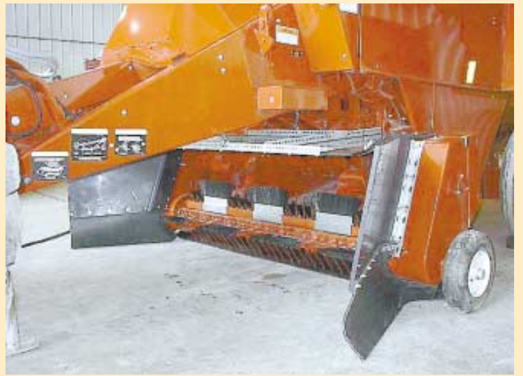
Abrasion-resistant nylon brushes mount behind tines on existing baler pickup. The brushes, which are staggered, sweep up leaves from smooth, paved surfaces.
