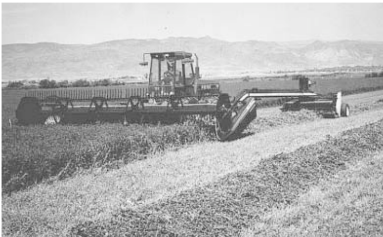
The Tufts mounted a 25-ft. MacDon 972 draper harvest header on front of their Ford Versatile Bi-Directional tractor and a Circle C crusher roller conditioner on back.
