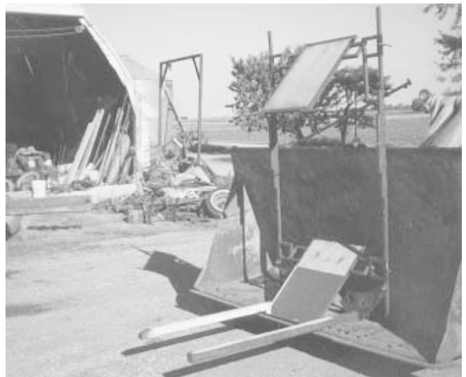
Steve Spiering mounted two mirrors on the bucket of his Deere payloader. The mirrors let him clearly see the forks from the cab.
