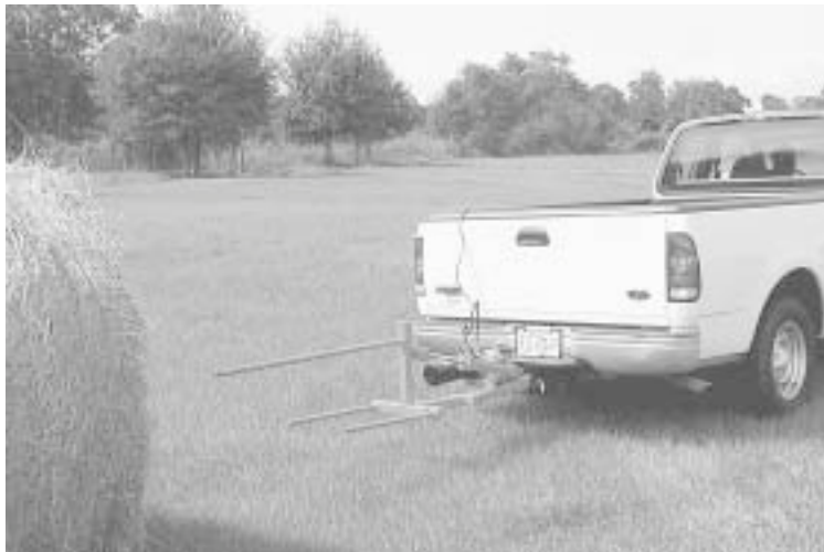
Round bale mover fits pickup receiver hitch. Bale spears are moved up or down by a self-contained electro/hydraulic motor. All operations are remote-controlled from the cab.
