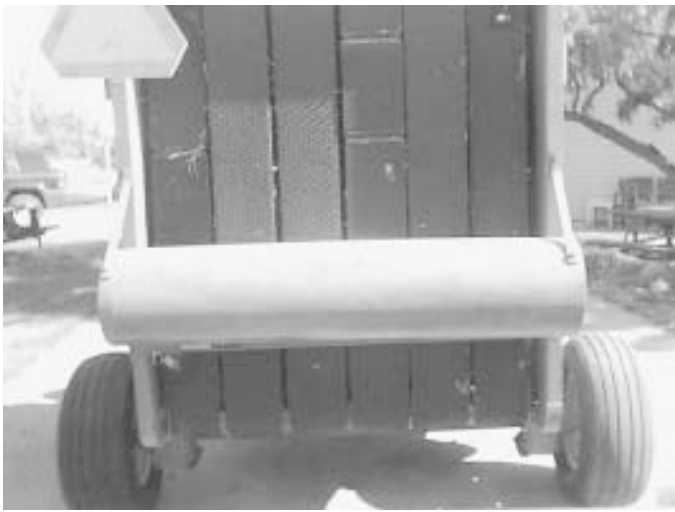
Dwaine Perrenot carries six extra rolls of twine inside a 10-in. dia. PVC tube that mounts on the back door of his Deere 430 round baler.
