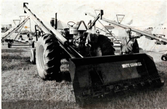
A dump hopper attaches to bottom of scoop to unload trucks and wagons.
