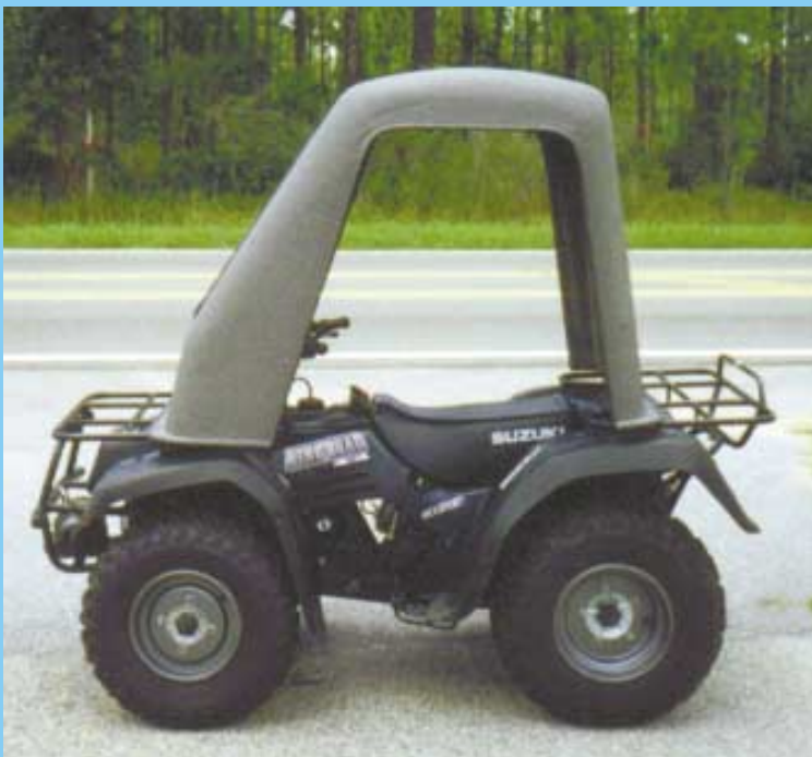
One-piece, fiberglass ATV enclosure bolts onto ATV’s front and rear racks.
